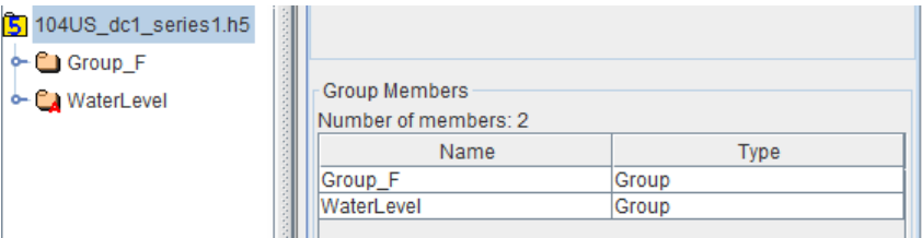
Figure E.1 - Typical HDF5 file (left) and its two groups, 'Group_F' and 'WaterLevel' (right)
