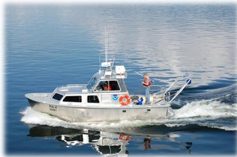
A typical small hydrographic launch used for near-shore and harbour surveys
