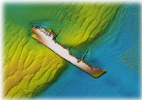
A wreck detected by side scan sonar
