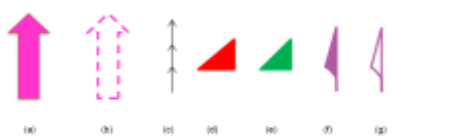
Figure 9.2 – Existing arrow types and approximate colours approved for use in ECDIS: (a) and (b) for traffic separation schemes, (c) for recommended (one-way) tracks, (d) and (e) for conical buoys,
