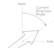
Figure 9.3 – Portrayal of the arrow's direction, based on the current direction
