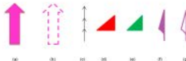
Figure 9.2 – Existing arrow types and approximate colours approved for use in ECDIS: (a) and (b) for traffic separation schemes, (c) for recommended (one-way) tracks, (d) and (e) for critical buoys,
