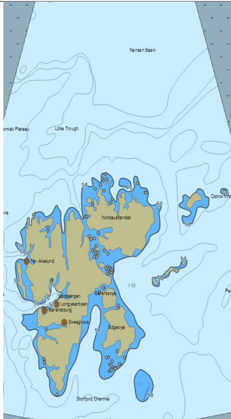
**TBD:** Note: Implementation of support for latitudes higher than  $85^\circ$  is an option for ECDIS. Polar projection is typically used for latitudes higher than  $85^\circ$ . ECDIS image in this example is based on polar projection
